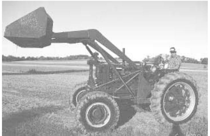
Front drive axle and traction grip tread tires are off an International Loadstar truck.
