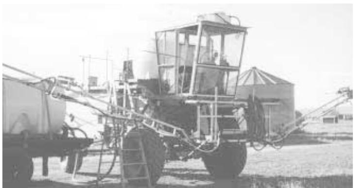
Combine's original header lift cylinders are used to raise and lower a commercial 3-section boom that mounts on front.
