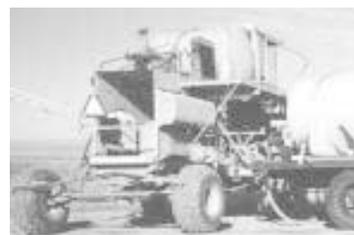
There's a 500-gal. tank mounted behind the cab and a 300-gal. tank mounted inside the thresher housing.
