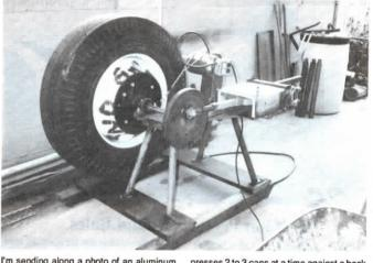
I'm sending along a photo of an aluminum can crushing machine I built out of miscellaneous parts. It consists of a large truck tire and wheel (weighs about 220 lbs.) that's turned at about about 70 rpm's by a 1/2 hp. electric motor salvaged from a washing machine. A friction roller mounted on the electric motor turns against the tire. The wheel turns a shaft connected to a round metal plate which drives a 5 by 12-in. piston with a 4 1/2-in. stroke. The piston com-
