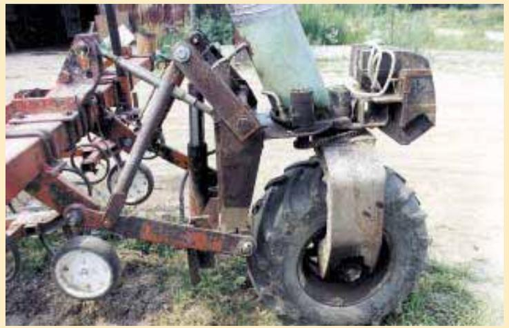
Front wheel mounts to a yoke made from 1-in. steel plate. A hydraulic motor chain drives a sprocket welded to a steel shaft to steer. Another motor direct-drives hub.
