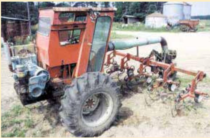
Air-cooled 50-hp. engine mounts behind the cab, which came off a combine. Operator has a wide open view of the up-front 4-row cultivator.
