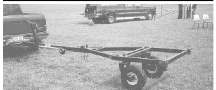
Easy-backing 15-ft. trailer is equipped with a pair of 8-in. caster wheels on back.
