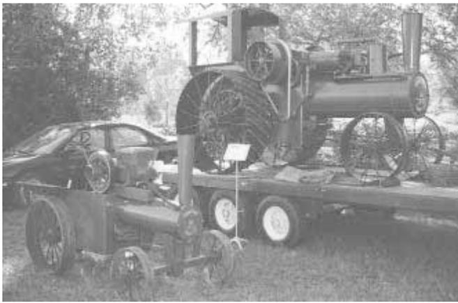
Tractor is powered by a 1936 Fairbanks Morse 3 hp water-cooled engine.
