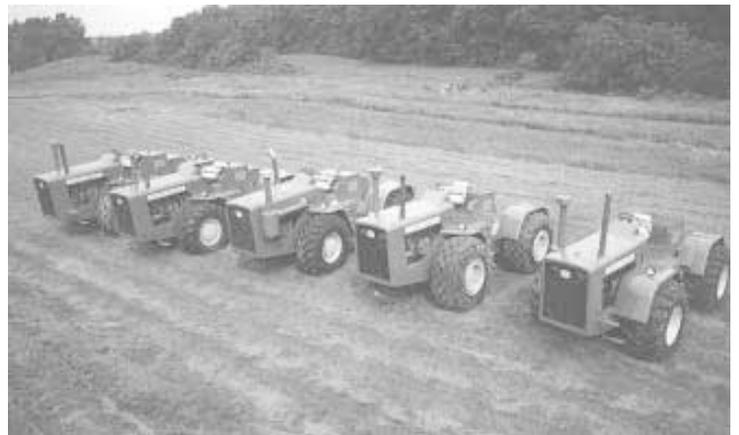
Kleiber’s five Deere 8020’s all needed a lot of restoration, including replacing electrical wires, cables, linkages and sheet metal and rebuilding brakes and seat platforms.
