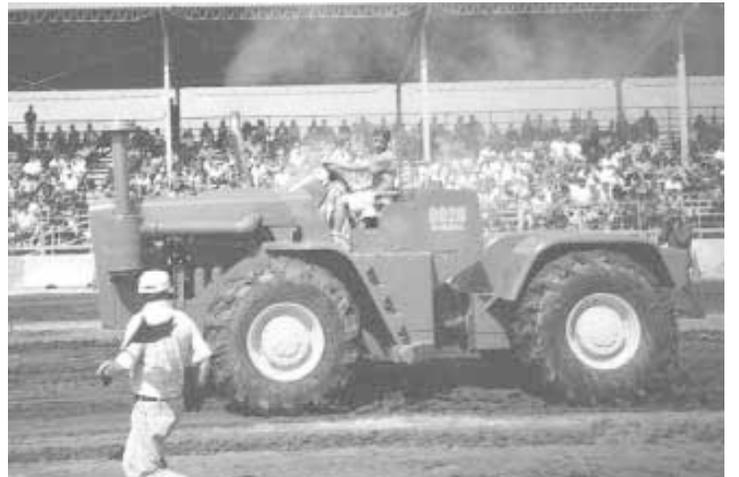
Modified for tractor pulls, this 8020 was repowered with a Detroit 871 turbo.
