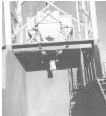
The tank stands on four legs fitted with weigh scales so cement and sand can be weighed as it's dumped into a mixing truck.
