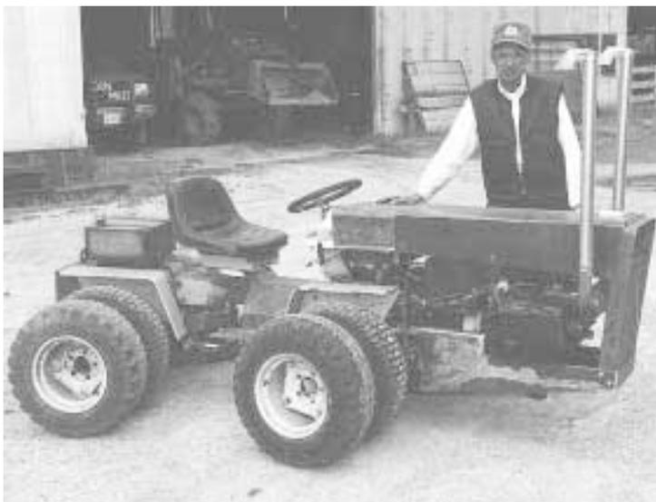
Tractor is powered by a 2-cyl. 18 hp Onan engine and has two Cub Cadet hydrostatic rear ends.
