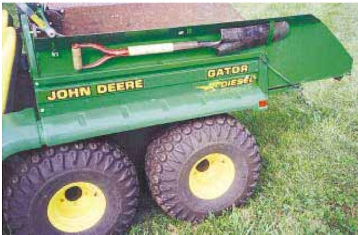
Made out of heavy 1/8-in. thick steel plate, the rock box bolts inside the Gator's existing box and can be easily removed when not needed.
