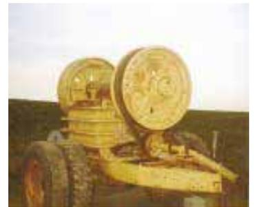
Rig is belt-driven by a 3-ft. dia. pulley that's counterbalanced by a large flywheel on back.
