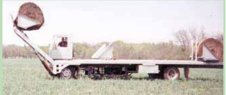
Photo shows how high bale loading arm can lift bale. Loading arm is fitted with bale forks and "bucket" that carries bales up onto the deck.
