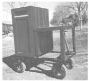
so I could mount my 5-in. vise on it. I made a hitch for the trailer out of 1 1/2-in. sq. tubing. It telescopes from 18 to 25 in. and folds underneath the table when not in use. The trailer rides on two 5/8-in. dia. steel shaft axles fitted with 3 by 10-in. pneumatic tires. I made my own front wheel swivel assembly so the rig trails my Honcho 4-WD ATV perfectly.
