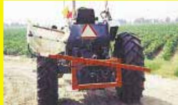
off a Red Ball sprayer and mounted it on a bar that fits our 3-pt. We set it to reach down into the ditch. For transport, it flips up behind the tractor. Works very well. (Harold Beville, 2958 E. County Rd. 378, Blytheville, Ark. 72319)
