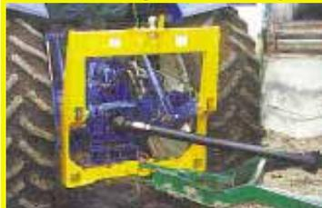
trolling vertical movement of the drawbar from the tractor seat. It uses an automatic latch that hooks up to, and releases from, the implement pin automatically, and it can pick the implement tongue up off the ground without the need for a mechanical jack. The pto can operate even when making a tight turn.
