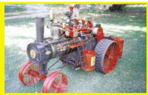
I worked on my mini steam tractor for three years. It's an exact scale replica of a 40 hp. Rumley Advance steam engine originally manufactured in 1912. It was a 225 hp., 2 cylinder tractor. My model has no castings in it. It's all hand made, machined or fabri-
