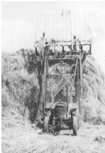
Stacker's winch was made from a Model T Ford rear axle.
