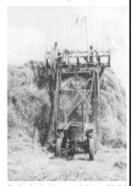
Stacker's winch was made from a Model T Ford rear axle.
