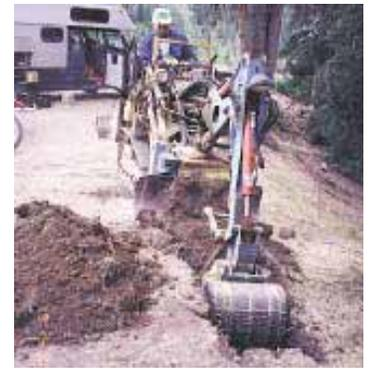
A variety of quick-release attachments can be used with the rig, including this front-mount, 18-in. wide backhoe.
