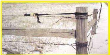
New fence stretcher weighs only 1 1/2 lbs. and consists of a ratchet attached to a seatbelt-type nylon strap that has a hand loop in it.
