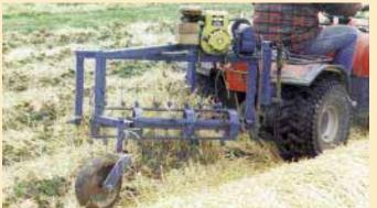
Mulch remover consists of spring tines welded to a small reel that's chain-driven at one end by a 3 hp motor.
