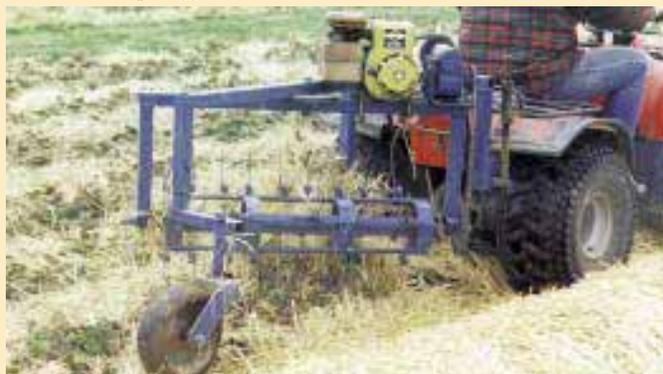
Mulch remover consists of spring tines welded to a small reel that's chain-driven at one end by a 3 hp motor.
