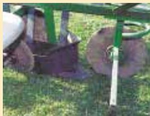
A no-till wavy couler cuts ground ahead of a V-shaped opener with a cultivator sweep on front.
