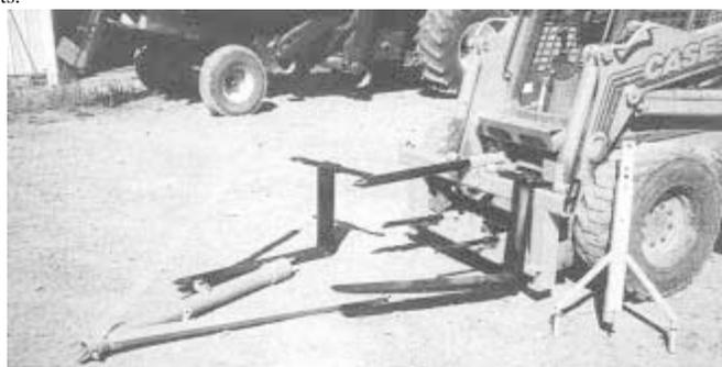
Bale spear, pallet forks, 5-ft. boom and drawbar can be used with the skid steer loader.
