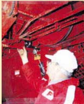
**Kit provides on-the-go mechanical adjustment for Case-IH Axial Flow combines from the late 1970's through 2188's built in 1993.**
