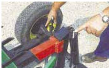
Back of rig has two indicators. One shows how much the scraper is raised and lowered; the other shows how much it's tilted.
