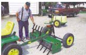
Box scraper is equipped with scarifier teeth positioned 8 in. ahead of blade.
