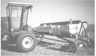
Cart raises up to 24 in. with a pair of 2 in. cylinders to make loading header easy.
