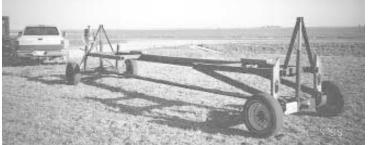
Hydraulic cylinders operate with a hand pump located on front of the cart.
