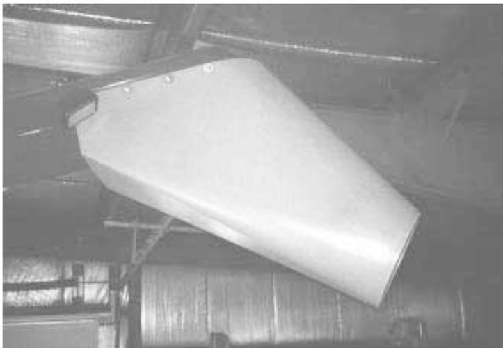
**Bolt-on spout drops grain about 3 ft. beyond end of auger, so tractors and grain carts don't have to get as close to combine.**
