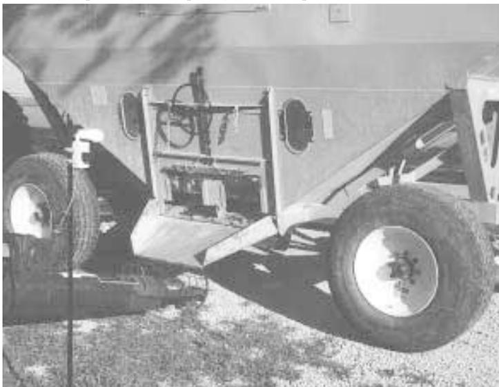
**Electronic eye "reads" light reflected from tape on side of wagon or truck, turning on bulb to alert driver.**
