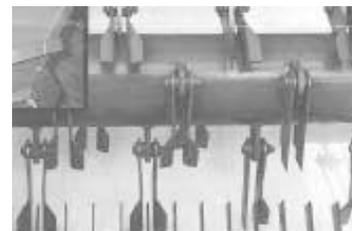
**Two models are available - one equipped with straight knives and the other with a bent hammer/straight knife combination.**
