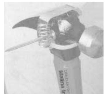
Device fits over the hammer head and is held in place with a nylon strap.
