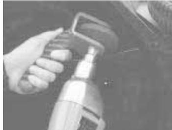
Sharpener fits into the drill like a bit. Makes it easy to hold and maintain the right sharpening angle.
