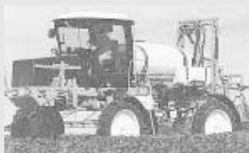
Most feature: radial piston wheel motors that "provide the most efficient transfer of power to the wheel available"; air spring suspension; 60 to 90-ft. self-leveling booms with tip breakaway protection.
