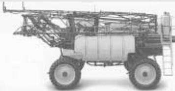
Features: Cummins engine; 60-ft. hydraulic-fold, front-mount boom.
