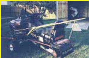
and is powered by a 3.5 hp Briggs and Stratton lawn mower engine coupled with a lawn mower transmission. The transmission chain drives a sprocket that powers the left wheel, making it effortless to move the snowmobile forward and backward and to turn it with the handle mounted on back.
