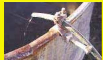
I welded an ordinary cable clamp to a curved "saddle" I cut out of a 2-in. section of pipe that fits over the lip of my tank. I welded a nut to one side of the saddle. A bolt screws into the nut to hold the hose securely to the lip of the tank.
