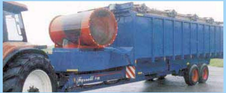
Fan sucks hot air through a large opening under the burner, then forces it through the trailer's perforated drying floor.
