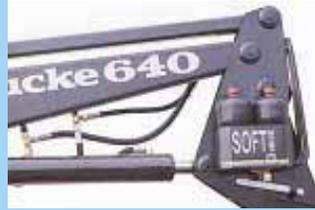
"Soft Drive" consists of two accumulator units.
