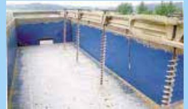
A series of equally spaced vertical augers move back and forth across trailer bed at 10-minute intervals to stir up grain.
