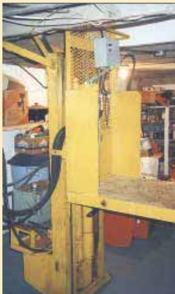
**A salvaged 3-ton forklift equipped with 6-ft. mast was used to build the elevator, which is powered by a 3 hp electric motor and 12 gpm hydraulic pump.**
