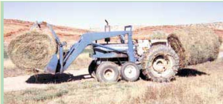
**Roden replaced the original 7.50 by 18 tires (shown here standing between tractor's front and rear wheels) with 11.00 by 16 ones mounted on heavy duty offset wheel rims.**
