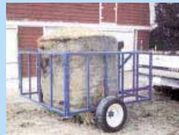
**A panel on back of the trailer is removed via two pins to load or unload the bale.**
