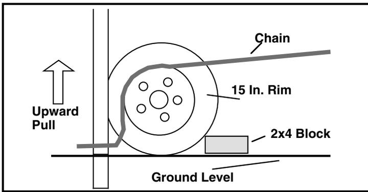
To pull a fence post, Trenary simply wraps the end of a piece of chain around the post and runs it over the top of a 15-in. car wheel rim.
