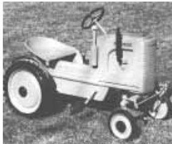
These custom-built pedal tractors are modeled after Deere L, LA, and LI tractors. Bodies are made from fiberglass, with three layers of resin and two layers of matting.
