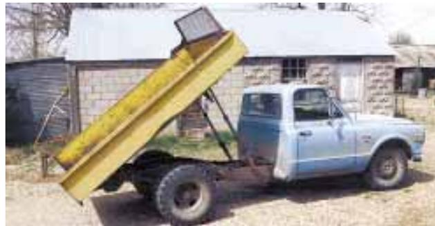
Ray fitted 1968 Chevy 1-ton pickup with home-built 10-ft. long steel bed. A pair of hydraulic cylinders are used to raise and lower the bed.
