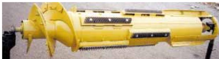
This rotor is out of a New Holland TR 70/TR 85 combine. Note spacing and depth of teeth on rasp bars.
