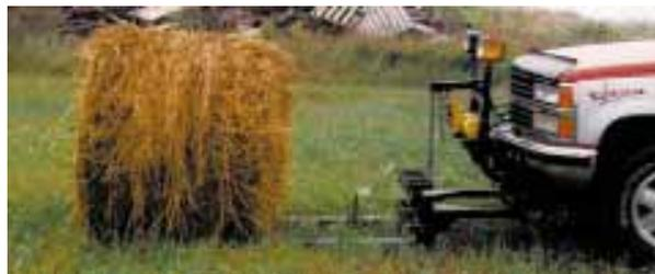
Two-pronged bale fork mounts on a rectangular steel frame that attaches to snowplow frame with two pins and a lift chain.
