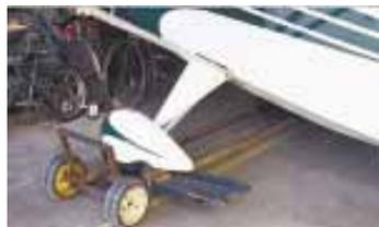
Ellis positions the plane's landing gear on the ramps and then pulls it inside by hand or with a garden tractor.
