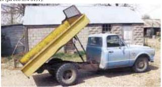
Ray fitted 1968 Chevy 1-ton pickup with home-built 10-ft. long steel bed. A pair of hydraulic cylinders are used to raise and lower the bed.
