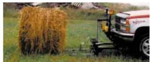
Two-pronged bale fork mounts on a rectangular steel frame that attaches to snowplow frame with two pins and a lift chain.
