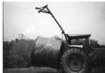
Schum made this 3-pt. boom to lift the rack up by the top ring and lower it over the bale. Raising the boom leaves room to carry a bale on tractor's 3-pt. hitch.
