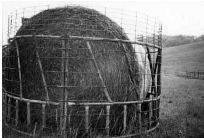
With feeder rack upside down, Schum welds 54-in. high wire combination panels onto the rings and slanted bars and cuts out two openings at each end of bale.
