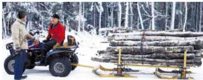
ATV-pulled bobsled is a scaled-down replica of an old-style, horse-drawn bobsled.
