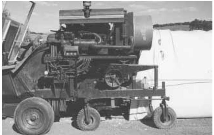
Bagger still has the original hydraulic-powered cable rewind system.
