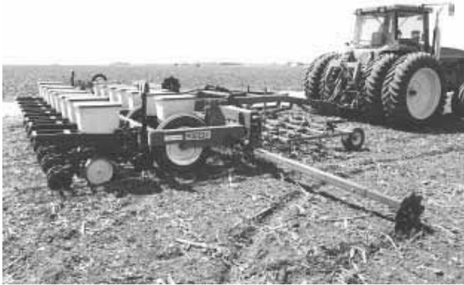
Follmer's 15-row, 15-in. double toolbar planter features seven row units on front and eight on back. A cultivator mounted ahead of the planter eliminates tracks.
