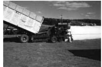
Brown added parts from several machines to the bagger, including a 220 cu. in. 6-cyl. gas engine off an International combine, which belt drives the bagger's rotor.
