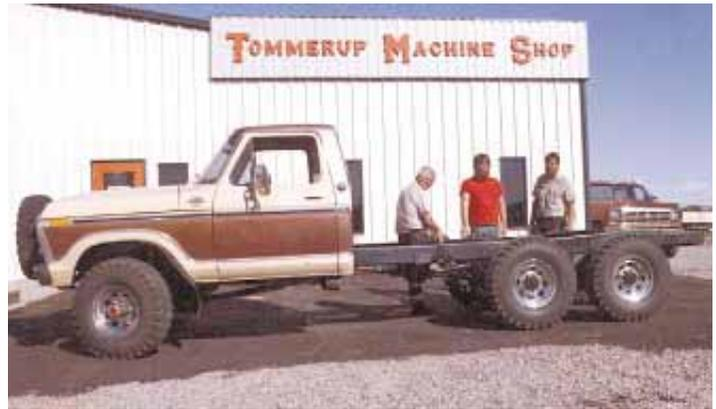
Hampton cut off the pickup frame about 3 ft. behind the cab and welded on a 12-ft. long frame he took from an early 1970s crew cab pickup. He fitted the new frame with the original rear axle and the rear axle off a 1973 Ford 3/4-ton 4-WD pickup.
