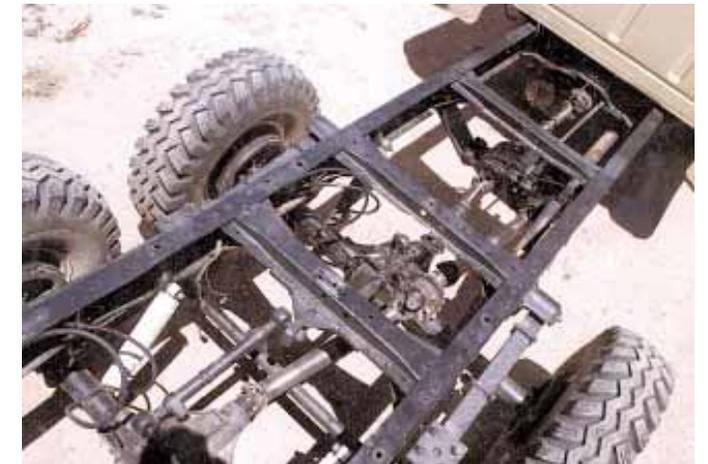
He mounted an extra transfer case 2 1/2 ft. behind the cab, positioned so it faces backward. A pair of driveshafts on the transfer case are used to power the mid and rear axles, with one driveshaft going to each axle.
