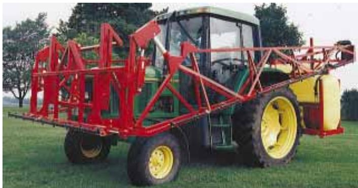
Front-mount boom lets you use the horsepower you've already got to do your spraying and, unlike a pull-type, eliminates wheel tracks that can damage narrow row crops.
