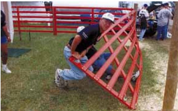
New fiberglass gate can be bent almost down to the ground but will straighten right back up.
