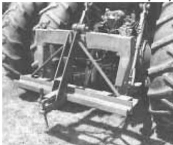
attachment on the 3-pt. hitch. It allows me to level my 24-ft. field cultivator, disc and other implements on the go, which is a time and back saver.
