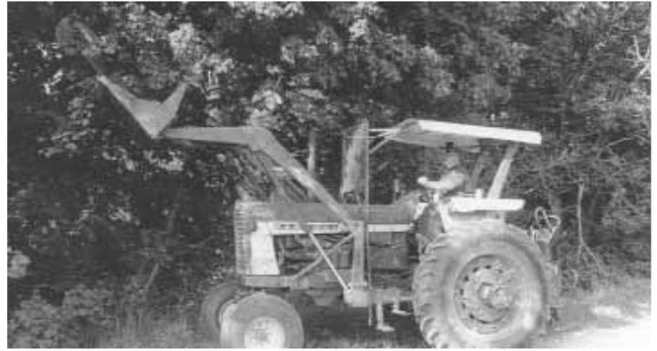
Hydraulic powered brushcutter saws through 3 to 4-in. dia. branches with ease, Brook says.
