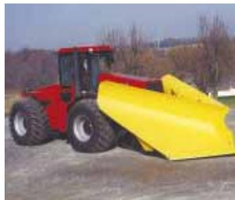
order to reduce wear. We use a Case-IH 7120 tractor that's equipped with an 11-ft. wide, 42-in. high blade to follow behind and clean up. The blade on that tractor can be angled left or right.
