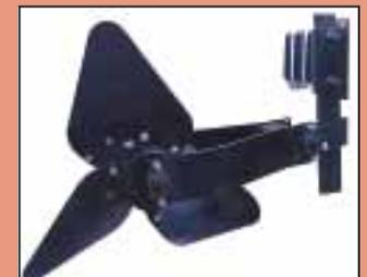
The "Prop" has three blades splayed out at a 45 degree angle from the hub. They dig little water-catching dams as they work through the soil behind ripper.
