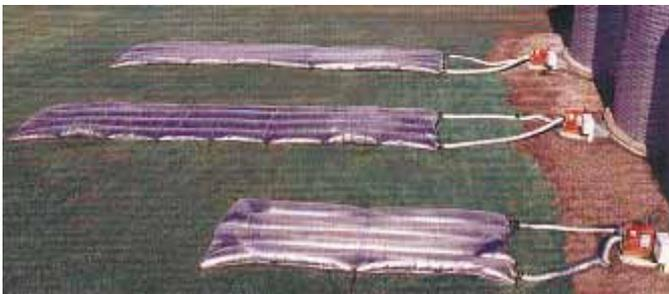
Plastic inflatable solar collector hooks up to the intake side of virtually any existing aeration fan. Air pressure moves air through the solar collector and into the bin.
