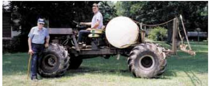
Minick used 3-in. channel iron to build a frame that supports a 300-gal. spray tank behind the seat.
