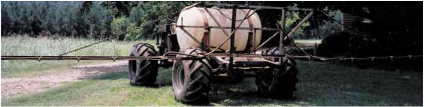
The 4-WD pickup was stripped down as much as possible to save weight and rides on 18.4 by 16 flotation tires, allowing it to float on top of ground without leaving deep tracks.
