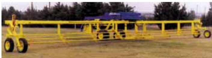
Shelbourne's 60-ft. pull-type stubble cutter is designed to cut down standing stubble left after harvest by the company's stripper header.
