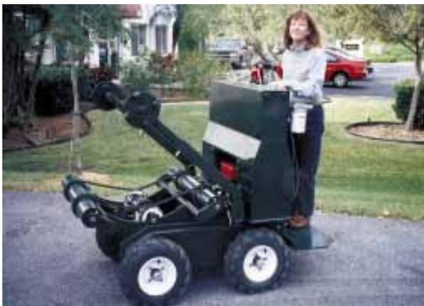
Operator stands on a platform behind a pair of hydraulically-operated clamp arms and a table that tilts forward to pick up a bale.
