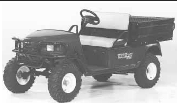
The Workhorse ST-350 mounts on 20-in. high turf saver tires and has an electric-operated dump bed. The two-passenger seat is made from fabric-backed vinyl.
