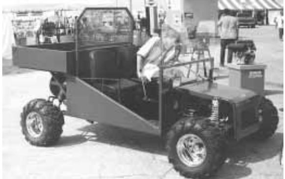
The 2-WD Sigby tractor mounts on 26 by 12 by 12-in. turf tires and has a 44 by 56-in. cargo bed. The wheels are powered by separate hydraulic motors.
