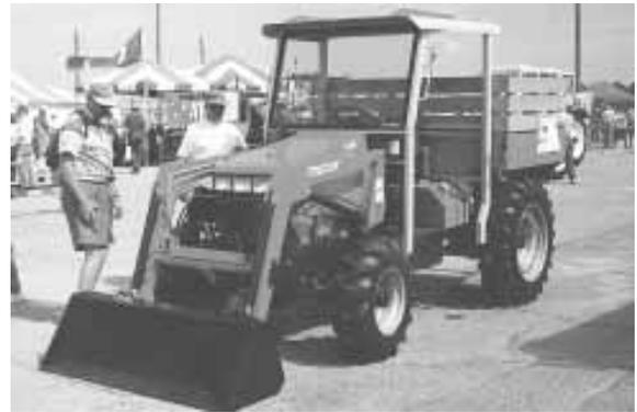
The T-4000 is equipped with a modular 3-pt. hitch and independent live pto that can be used either at front or rear, and a 2,000-lb. capacity hydraulic-operated dump box.
