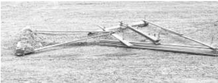
Worn cutting edges off road graders are bolted together to form the leveler.
