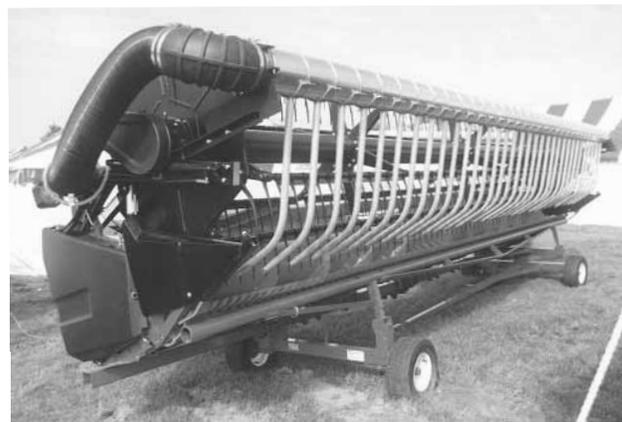
Reel uses the latest Crary gearbox-driven fan and out-front Keho-style manifold for more airflow with less horsepower.
