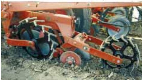
The open wheels don’t compact soil like solid wheels, preventing crusting and making it easier to close the seed furrow.
