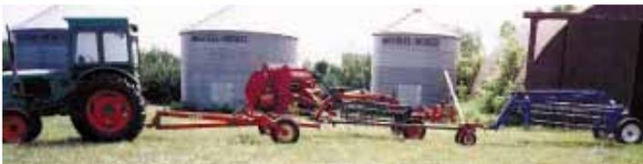
Double rake hitch allows White to pull two 9-ft. side-delivery rakes at a time. He built it out of an old 22-ft. field cultivator.
