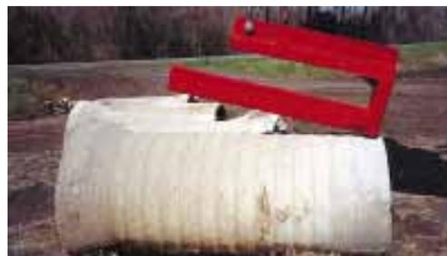
Pipe mover is made of two pieces of square steel tubing - the bottom one is 35 in. long and top one 28 in. long.
