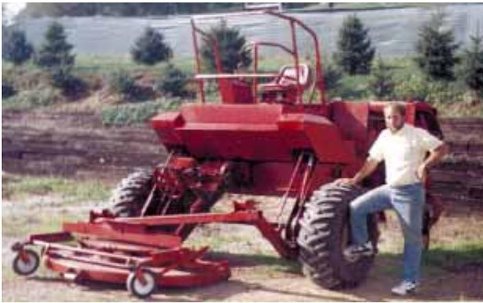
Heavy duty 6-ft. mower deck mounts in place of swather's original header and is driven by a gearbox off the swather's existing horizontal driveshaft.
