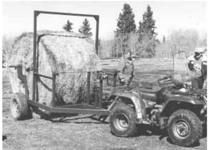
Trailer is operated by hand winches, eliminating batteries and hydraulics.
