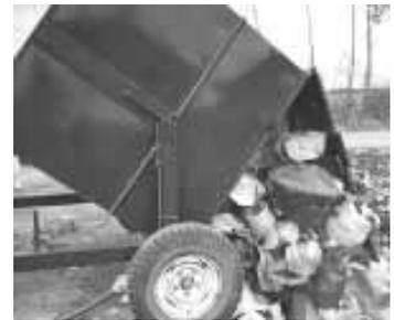
Bale spears, dump box, and rolling feed drum mount on a pair of uprights (above). A 31-in. wide rolling feed drum unloads grain on the ground (below).
