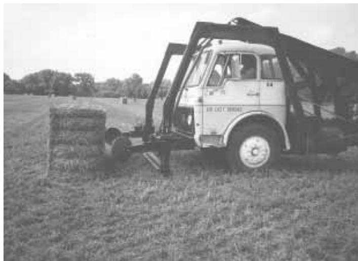
**Clamps on bow-shaped loader arms are fitted with 1 1/2-ft. dia. disc blades.**
