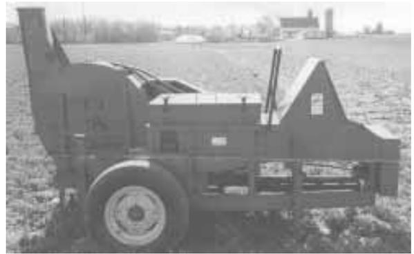
Pto-driven silo blower is equipped with two 9 1/2-in. dia. rollers that crack kernels to boost nutritional value of feed.
