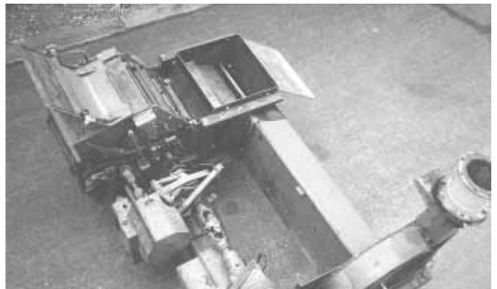
The company also sells a kit for installing a roller mill on a pull-type silage harvester. The blower is moved back 14 in. in order to make room for the rollers, which mount right behind the cutter knives. They recommend removing half the knives in order to offset the increased horsepower requirement. Harvester is shown here with header removed.
