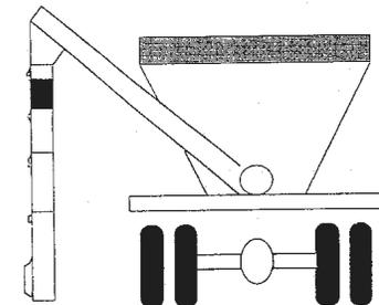
**Plastic telescoping downspout will outlast conventional downspouts by 5 to 10 years.**
