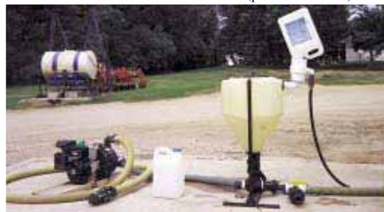
Rinse system installs on the side of the 15-gal. chemical induction tank plumbed between 1,500-gal. water tank and 5 hp pump.
