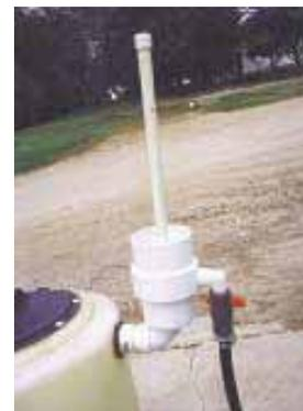
A 17-in. long piece of 1-in. dia. PVC pipe extends upward and has holes drilled in it at regular intervals. Empty containers slip over the top of pipe, which is fitted to an elbow that extends out to the side. The elbow hooks up to a water hose. The rinse water."
